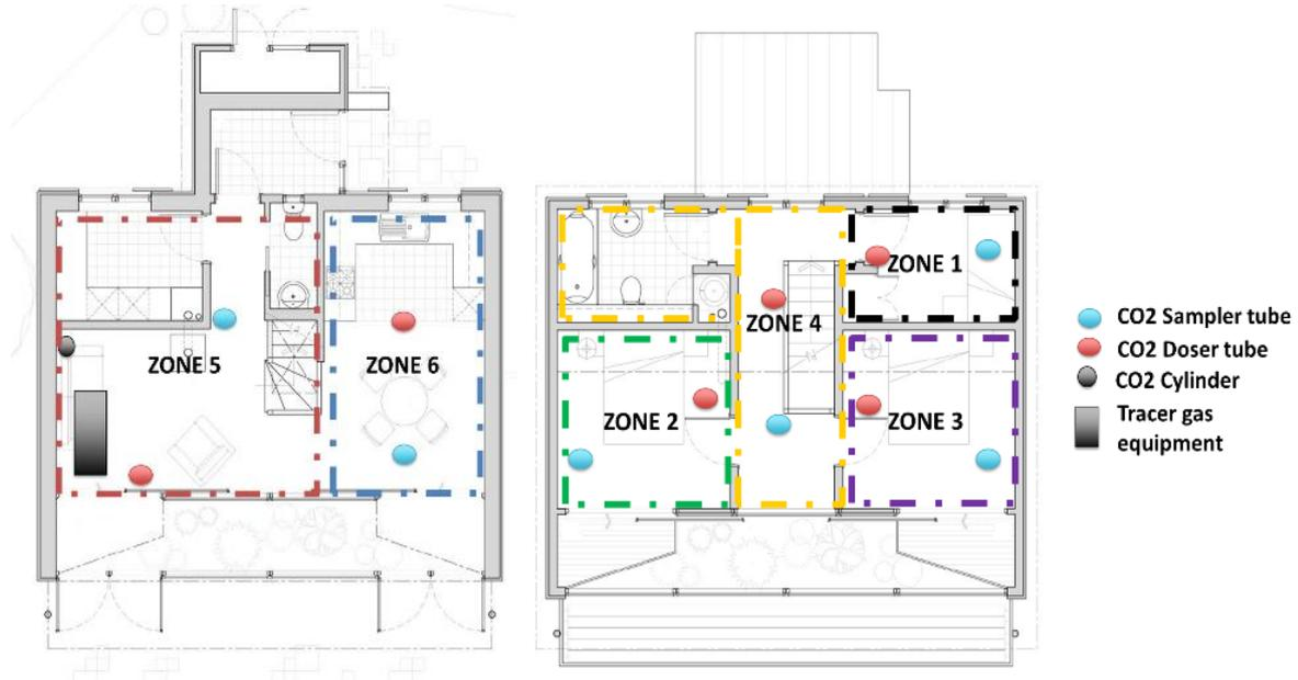
Figure 2. Floor plans of the case study house and location of equipment setup
