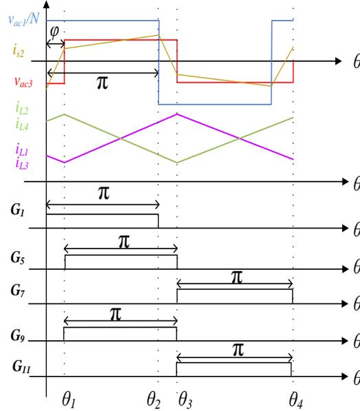
Figure 2: ABAC modulated with SPS using the classical switching pattern. Note that  $G_1$ - $G_{12}$  drive T<sub>1</sub>-T<sub>12</sub> in Figure 1 with  $G_4=G_1$ ,  $G_2=G_3=not(G_1)$ ,  $G_6=not(G_5)$ ,  $G_8=not(G_7)$ ,  $G_{10}=not(G_9)$  and  $G_{12}=not(G_{11})$
