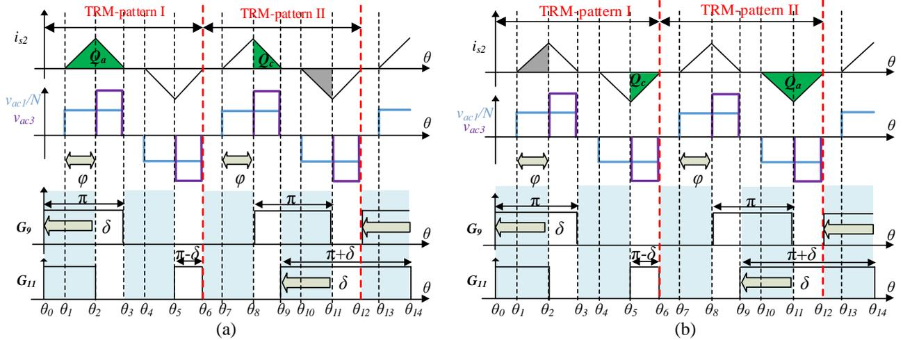
Figure 6: Balance charging illustration for (a) clamp capacitor  $C_3$  and (b) clamp capacitor  $C_4$  using TRM with the proposed alternated switching pattern.
