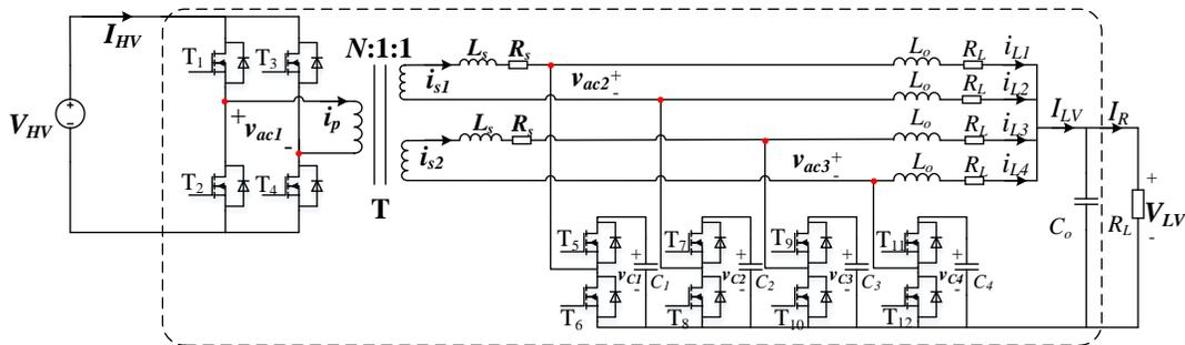
Figure 1: Circuit diagram of the ABAC converter.
