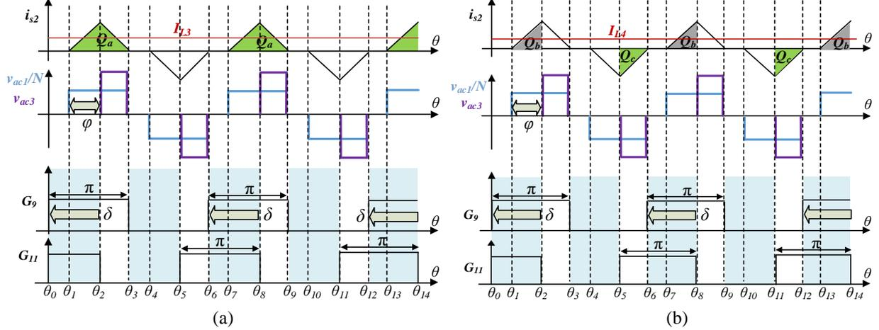
Figure 5: Asymmetrical charging using TRM with switching “pattern I” for clamp capacitors (a)  $C_3$  and (b)  $C_4$ .
