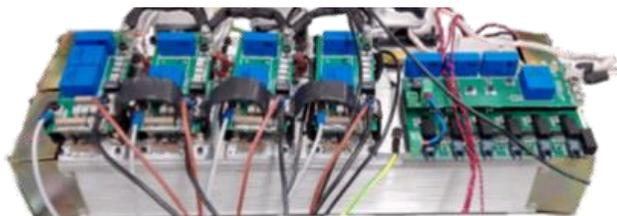
Figure 14: The 10kW ABAC experimental prototype
