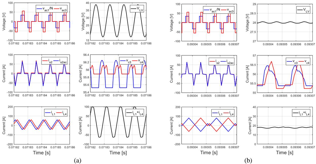
Figure 10: Simulations using TRM with (a) the classical switching pattern (synchronously switched secondaries) and (b) the proposed switching pattern under  $P=1\text{kW}$ ,  $V_{HV}=170\text{V}$  and  $V_{LV}=28\text{V}$ .
