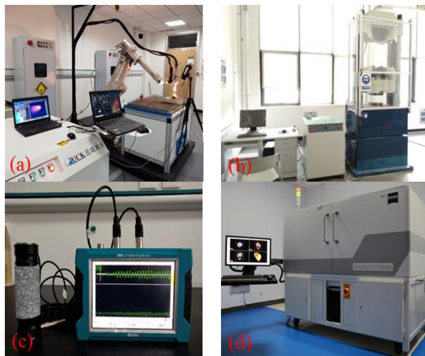
Figure 1. Devices used in experiments: (a) laser system, (b) electro-hydraulic testing servo machine, (c) ultrasonic tester, (d) X-ray micro-imaging system.
