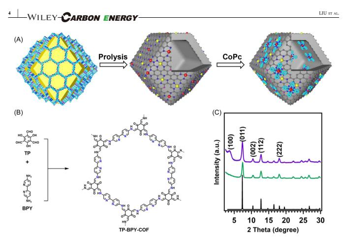
**FIGURE 1** (A) Synthesis of COF@MOF<sub>800</sub>-Co from COF@MOF. (B) Synthesis and structure of TP-BPY-COF. (C) PXRD patterns of COF@MOF (purple curve) and ZIF-8 (green curve) and simulation of ZIF-8 (black curve). COF, covalent–organic framework; MOF, metal–organic framework; PXRD, powder X-ray diffraction.
