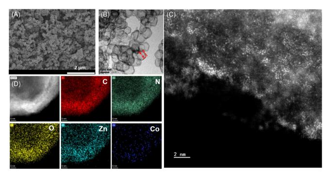
**FIGURE 2** (A) SEM image, (B) TEM image, (C) HAADF-STEM image, and (D) EDX-mapping images of COF@MOF<sub>800</sub>-Co. COF, covalentorganic framework; EDX, energy-dispersive X-ray spectroscopy; HAADF-STEM, high-angle annular dark-field scanning transmission electron microscopy; MOF, metal–organic framework; SEM, scanning electron microscopy; TEM, transmission electron microscopy.
