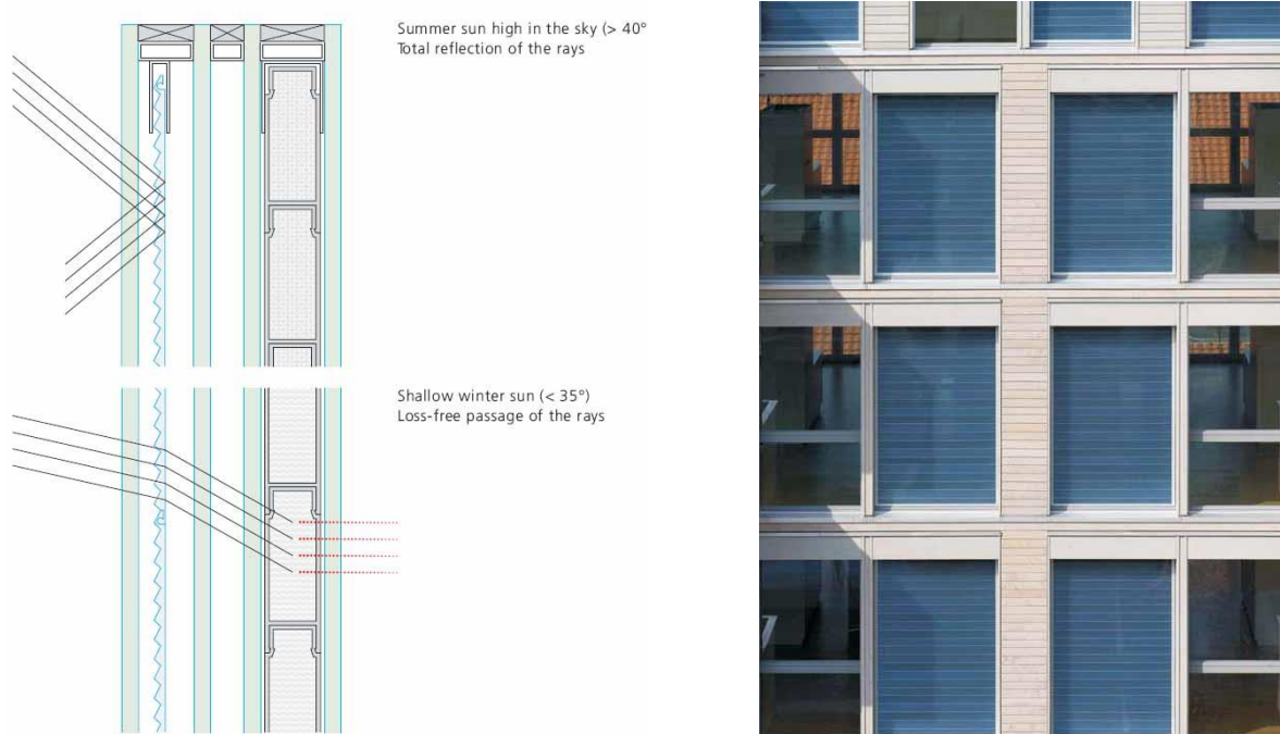
Fig. 5 Example of triple glass component. The prismatic panel reflects the radiation during summer and instead allows the heating of the thermal storage module (PCM in a polycarbonate box) in the winter season. The whole system, which looks like a translucent window, has a thickness of 80 mm, a thermal transmittance of 0.48 \text{ W/m}^2\text{K} and a light transmission coefficient that can reach up to 45% (GlassX AG technical documentation - www.glassx.ch ).
