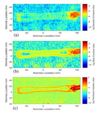
**Figure 1.** (a) Gaussian curvature map, (b) mean curvature map, c) prominence variation map of the  $16^{th}$  layer of a failed build with debris discovered on the right-hand side of the part. This tensile test piece was printed at 165 °C, 17 W laser power with a laser scan speed of 2500 mm/s and a hatch spacing of  $250 \mu m$ .
