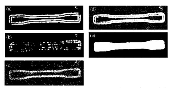
**Figure 4.** (a) mean curvature mask (b) Gaussian curvature mask (c) prominence variation mask after binarizing surface analysis maps based on Otsu's thresholding. (d) the result of a combination of three initial masks which represent the shape of part (e) the final mask is created after implementing the image processing methods of erosion and dilation.
