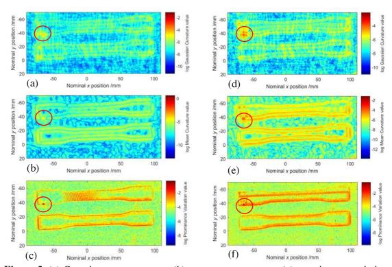
**Figure 3.** (a) Gaussian curvature map, (b) mean curvature map, (c) prominence variation map of the 19<sup>th</sup> layer where a surface protrusion, as marked with a red circle, on the left side of the top part. (d) Gaussian curvature map, (e) mean curvature map, (f) prominence variation map of the 28<sup>th</sup> layer where the observed surface protrusion is larger and in the same region of the top part.
