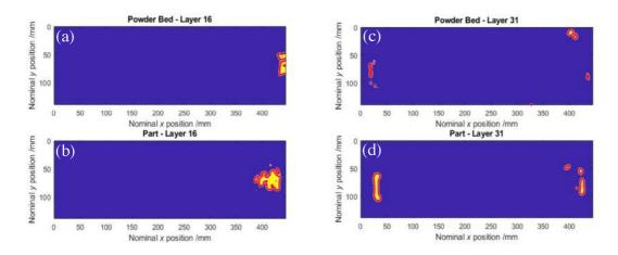
**Figure 8.** (a), (b) Separate analysis of the powder bed and the part where debris is observed on the 16<sup>th</sup> layer. (c), (d) Separate analysis of powder bed and the part where warping is observed on the 31<sup>st</sup> layer.
