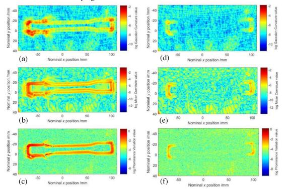
**Figure 2.** (a) Gaussian curvature map, (b) mean curvature map, (c) prominence variation map of the final sintered layer (30<sup>th</sup> layer) of a successful build with warping on both ends of the part. (d) Gaussian curvature map, (e) mean curvature map, (f) prominence variation map of the 40<sup>th</sup> layer of a build with the continuing effect of warping on both ends of the part.
