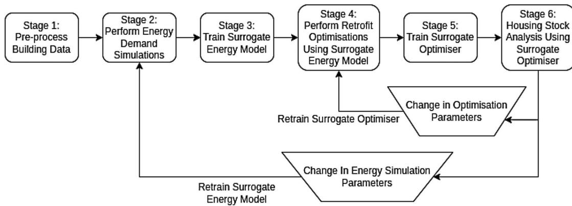
**Figure 1.** High level process flow diagram of method.
