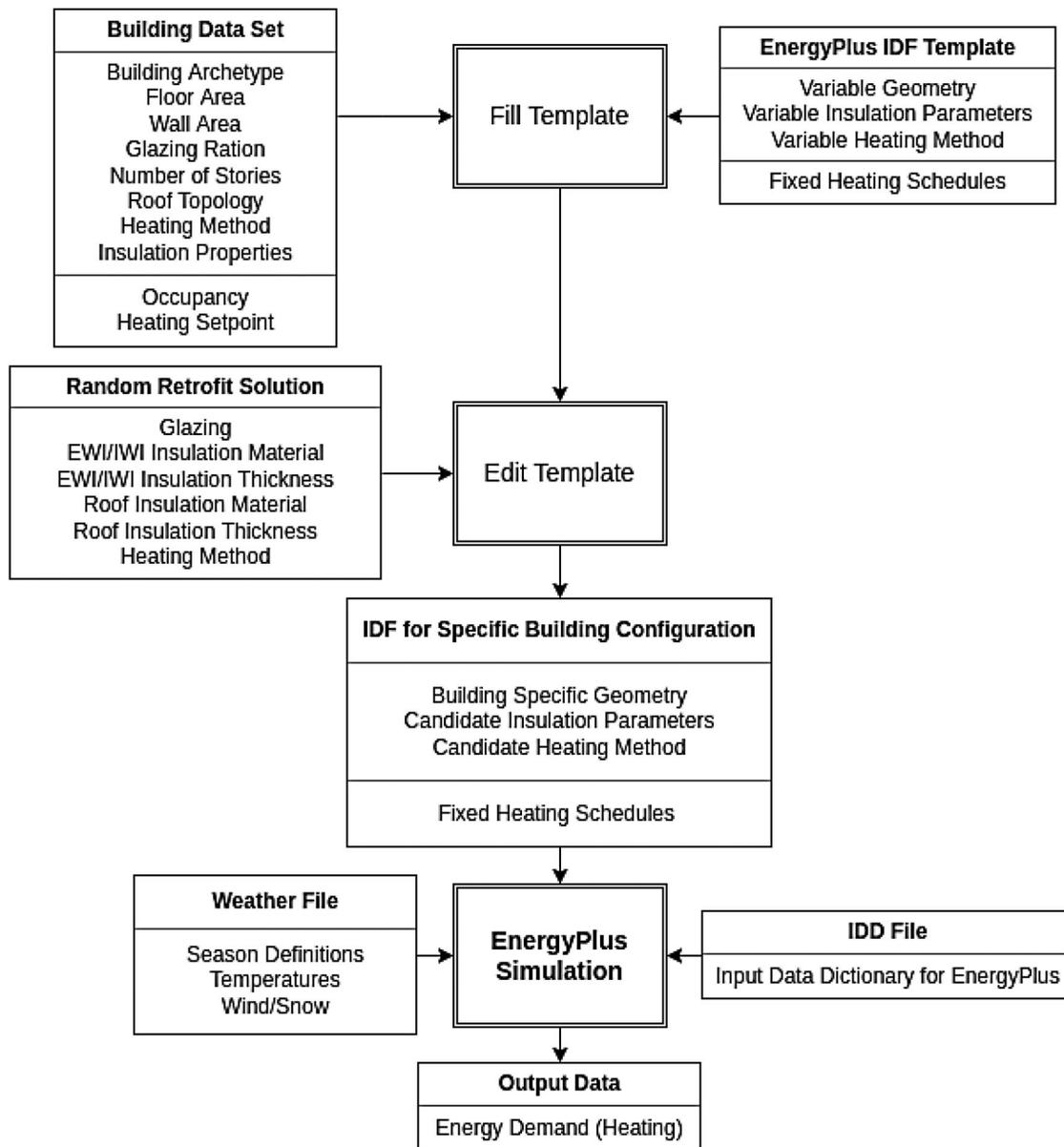
**Figure 2.** Conceptual data flow of single dwelling simulation during heating demand data generation stage (Stage 2).
