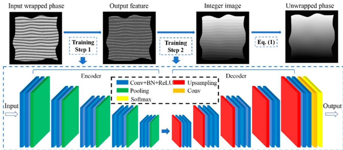
**Figure 6.** The workflow of the method proposed by Liang *et al* [140] showing the network architecture for phase unwrapping (Reproduced from [140]. CC BY 4.0.).
