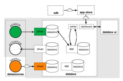
Fig. 1. Databox platform architecture
