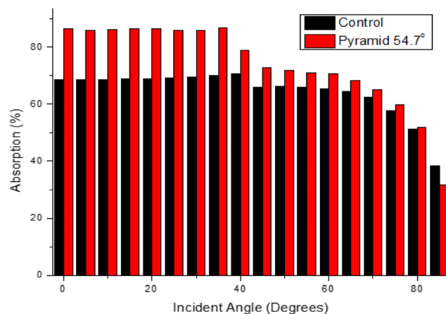
Fig. 4 Dependence of absorption on incidence angle of light of wavelength 540 nm for planar control and pyramids of side wall angle 54.7^\circ
