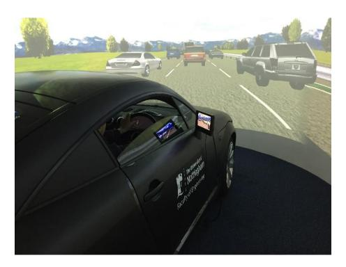
Figure 1: Medium-fidelity fixed-base Driving Simulator
