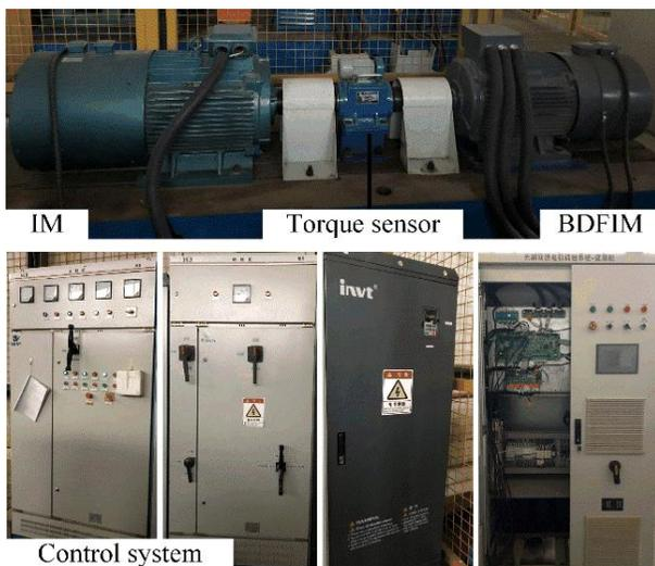
Fig. 11. The experimental platform.
