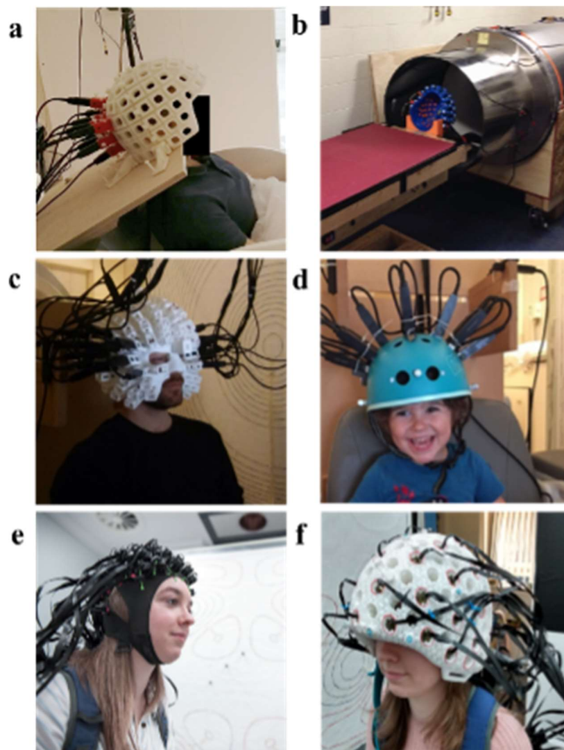
Fig. 4 The evolution of the helmet design: Photographs of a) a static, 3D-printed helmet (Iivanainen et al., 2020), b) a fixed 3D-printed helmet with moveable sensor holders to conform to different head shapes (Nardelli et al., 2020), c) a whole-head 3D-printed personal scanner-cast (Barry et al., 2019), d) a children's bike helmet (Hill et al., 2019), which has been modified to hold OPM sensors, e) a flexible, EEG-like cap (Hill et al., 2020), and f) a generic 3D-printed helmet based upon averaged adult MRI scans (Hill et al., 2020)
