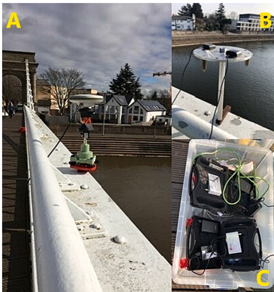
Fig. 17. A: Leica AS10 antenna & reflective prism underneath the GNSS antenna mounted at the midspan of the bridge, B: Two low-cost patch antennas with the same azimuth orientation at the midspan of the bridge, C: Low-cost GNSS receivers, raspberry pi models and power banks connected to the patch antennas in B.
