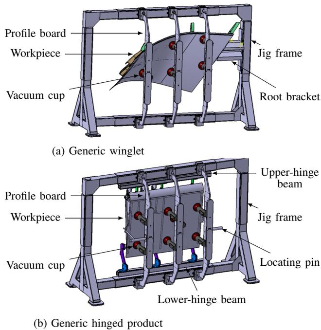
Fig. 1: Reconfigured jig for two different products
