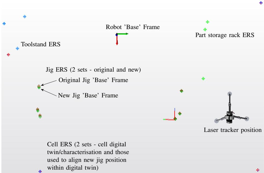
Fig. 9: Workstation layout captured by ERS points
