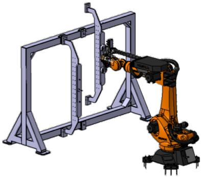
Fig. 3: Pick and place process: Robot load and unload profile boards onto the jig frame
