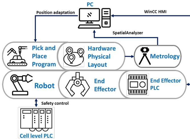
Fig. 8: Communication in testing cell
