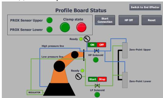
(b) Profile board connection HMI control
