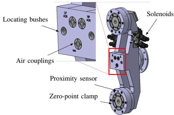
Fig. 5: Pick and place end effector with detailed service interface block
