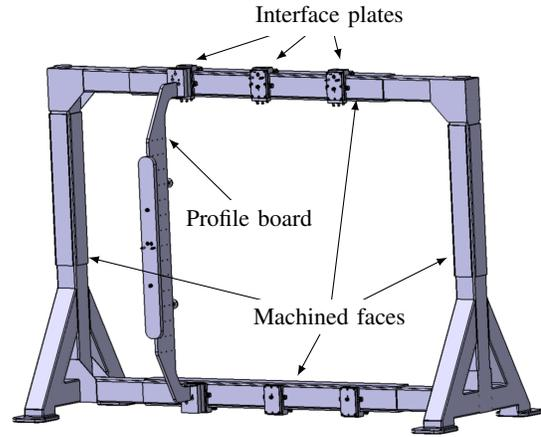
Fig. 4: Jig frame machined faces and interface plates mounted
