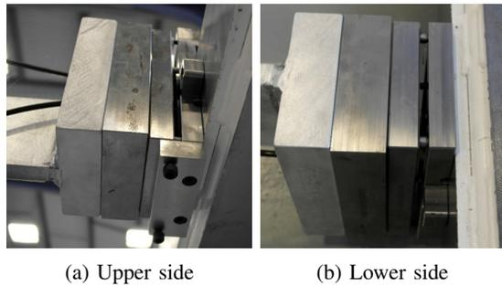
Fig. 11: Successful pick and place engagement after the jig position adaption
