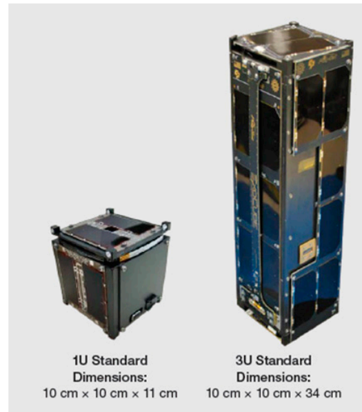
Figure 4. 1U and 3U CubeSat developed by CalPoly [24].
