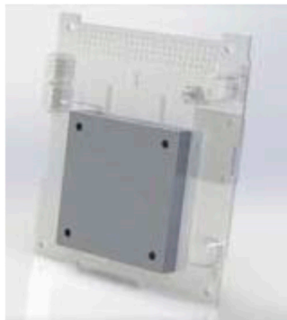
Figure 28. 2100 J CubeSat Thermal Storage Unit [46].
