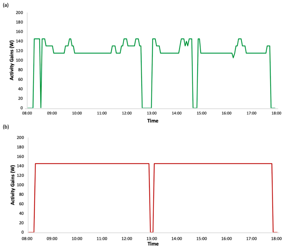
Fig. 4. (a). Example of an actual occupancy heat gains profile for a typical office day compared to (b). A typical static occupancy heat gains profile [62].
