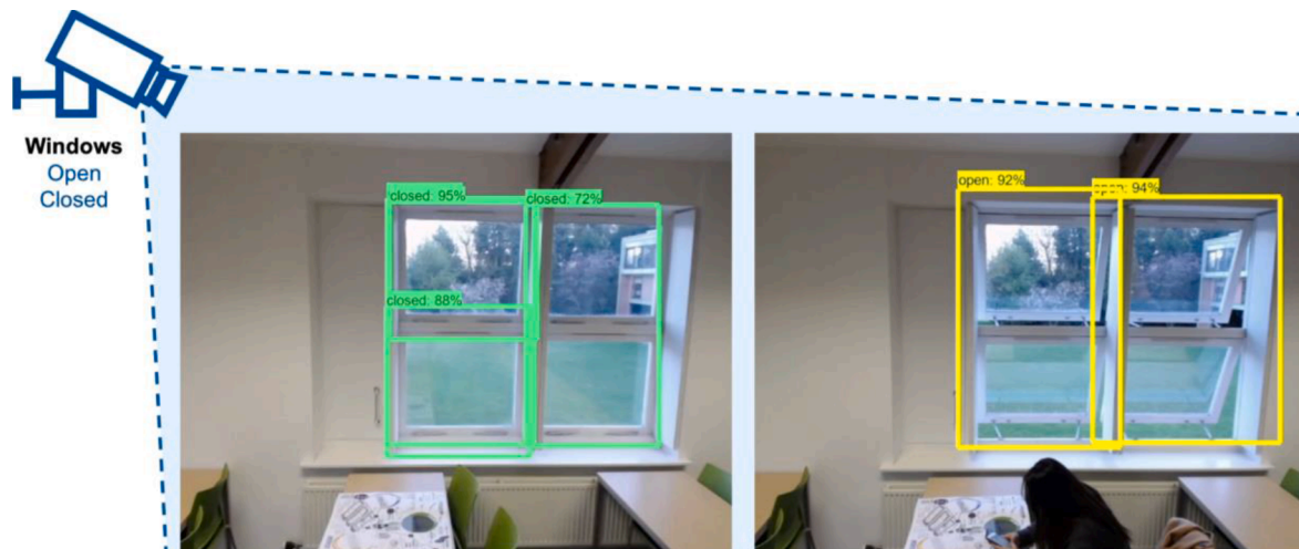
Fig. 8. An example application of an AI vision-based approach for window detection within an indoor environment. Refer to Video 2 to view an example of the detection and recognition.
