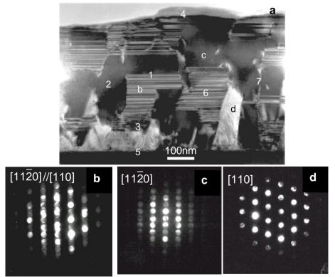
**Figure 1**. Focused probe diffraction patterns obtained from the areas labelled in (a) the bright field image for (b) a region containing stacking faults; (c) the wurtzite  $GaN < 11\overline{2}0 > matrix$  and (d) a zincblende GaN < 110 > grain.
