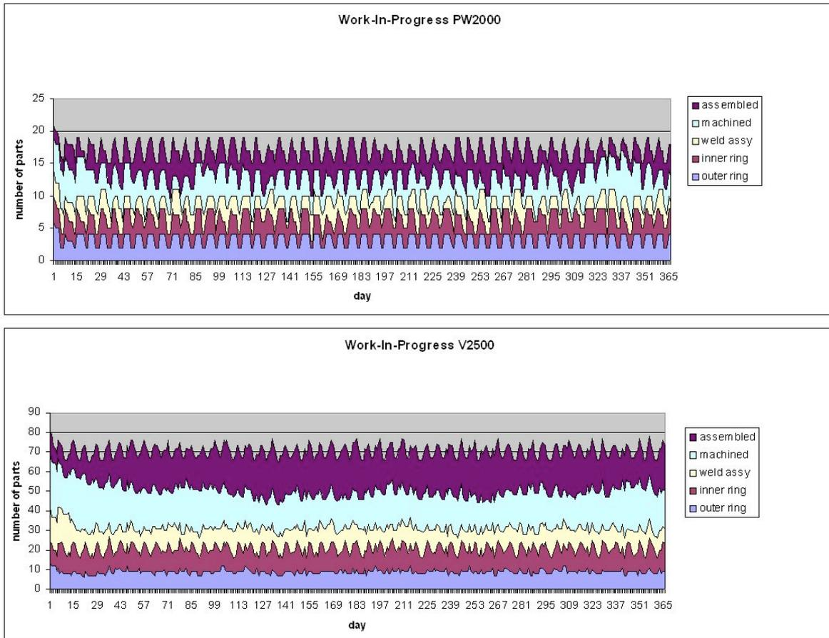
Figure 54: WIP levels observed, with quality problems in a 'push' system
