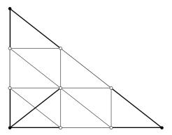
Fig. 2: A refined reference element of a mesh  $\mathcal{G}_m$ , where the black dots are the "father" nodes and the white dots are the "children". The thick lines link the children to their fathers.
