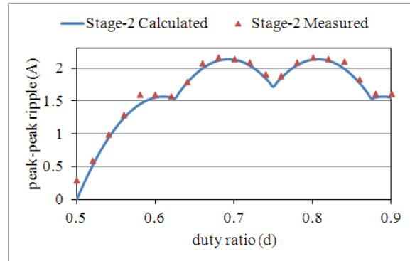
(b) Peak-to-peak ripple in stage-2 channel current
