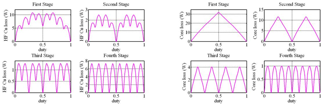
(a) High frequency Copper loss in the magnetic components
