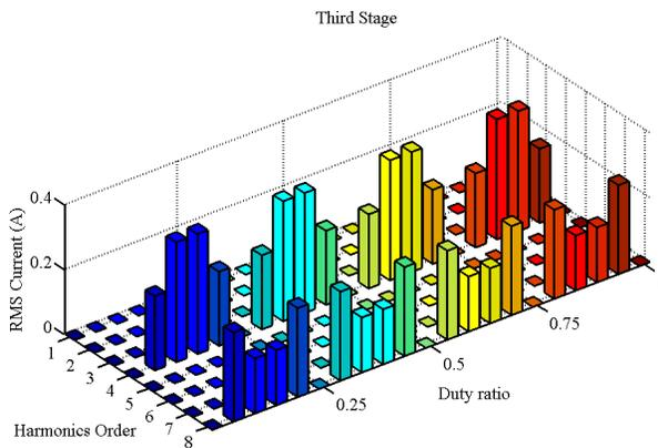
(c) Harmonics components in the stage-3 current
