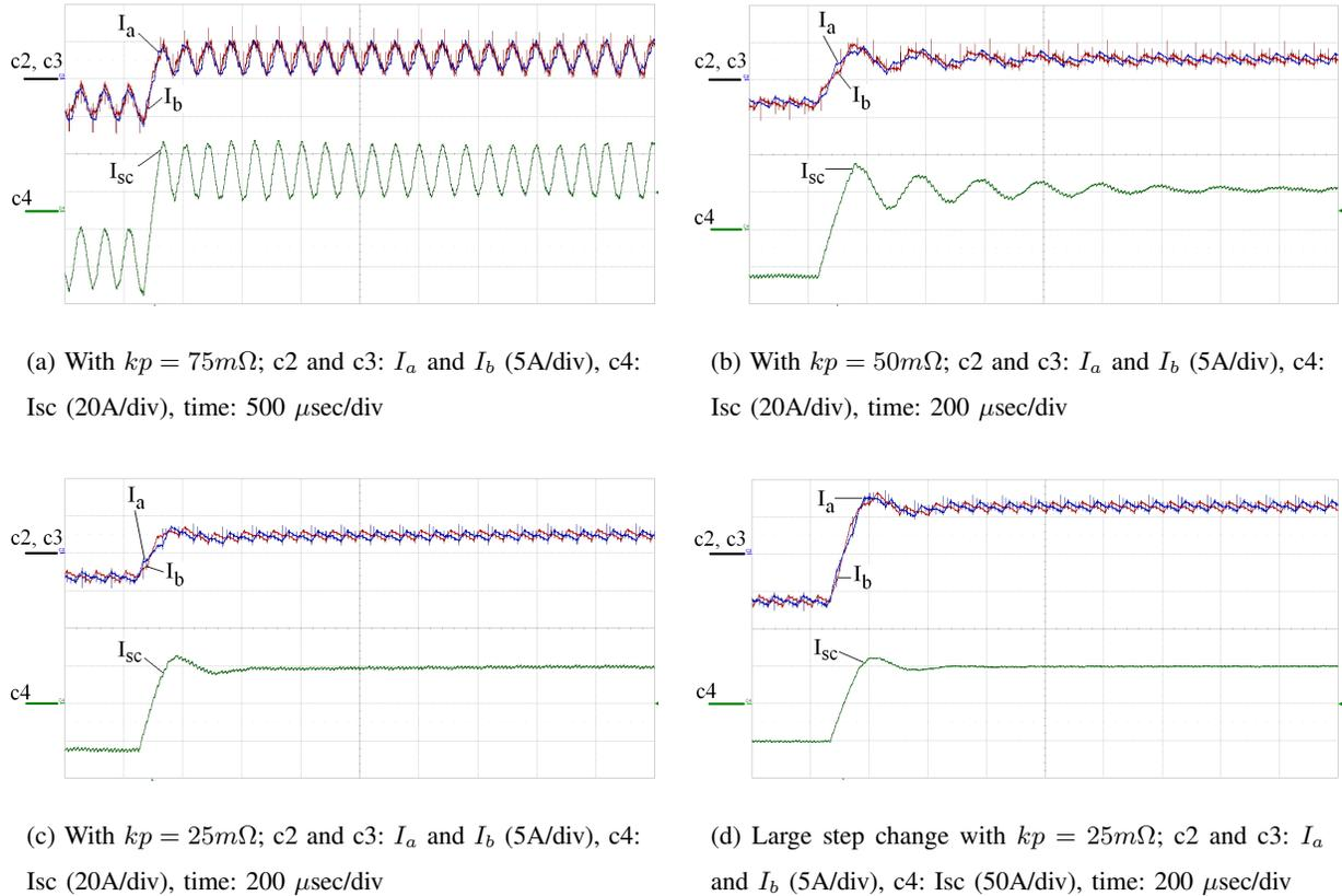
Fig. 12. Measured transient response with various controller gains
