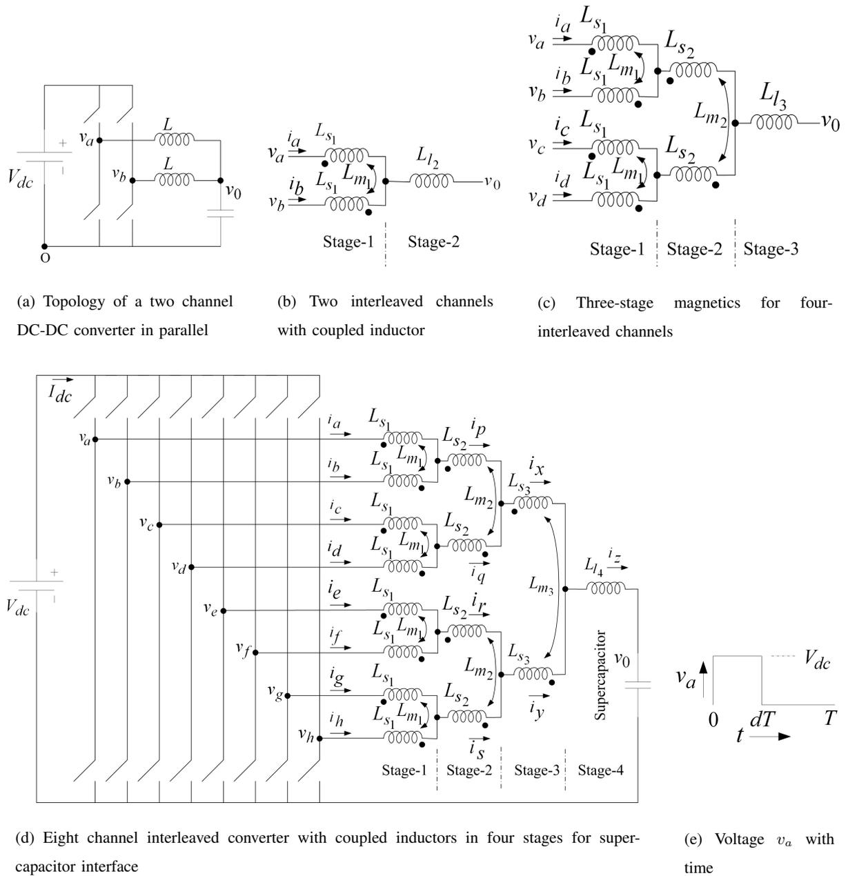
Fig. 1. Interleaved DC-DC converter topologies
