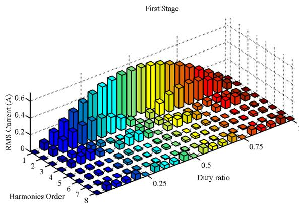
(a) Harmonics components in the stage-1 current
