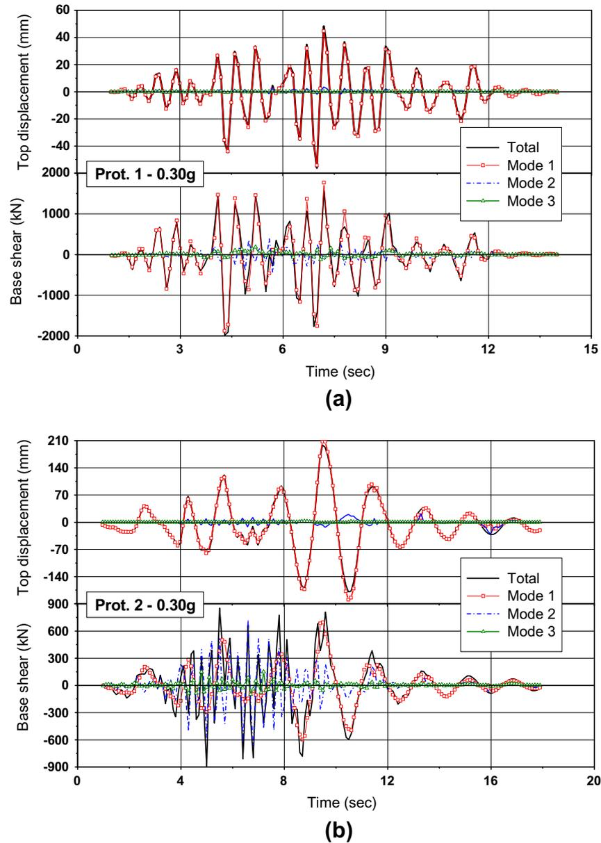
**Fig. 19.** Modal contribution response history of the 3-DoF system-in terms of roof displacement and base shear-to the applied ground motion of 0.30 g, for: (a) Prototype 1. (b) Prototype 2. (c) Prototype 3. (d) Prototype 4.
