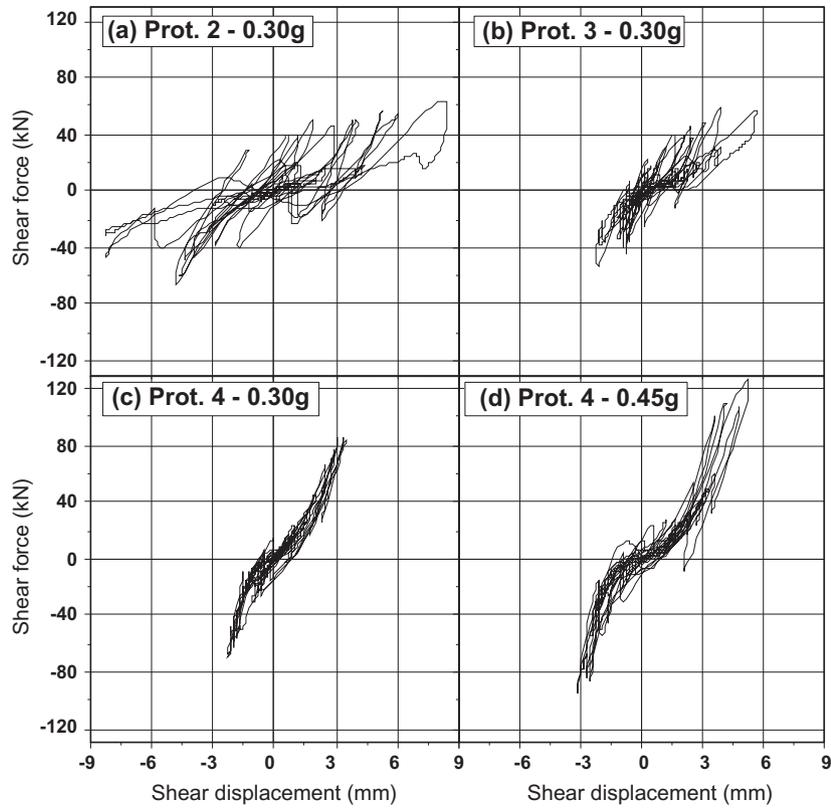
**Fig. 11.** Joint shear force versus the joint slip loops for an external beam-column joint (J13) of the third floor of: (a) Prototype 2 at PGA 0.30 g. (b) Prototype 3 at PGA 0.30 g. (c) Prototype 4 at PGA 0.30 g. (d) Prototype 4 at PGA 0.45 g.
