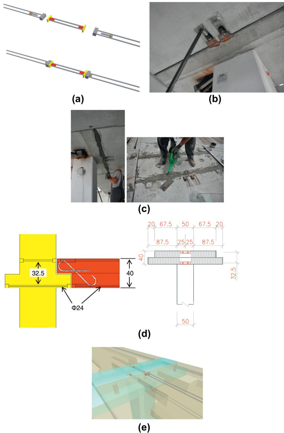
**Fig. 8.** (a) Loosen and activated connection system in its bare configuration. (b) Activation of the loosen bolts to provide continuity to the longitudinal bars crossing the beam–column joint. (c) Filling the gaps in the joints with mortar. (d) Detail of an emulative beam–column joint. (e) Three-dimensional representation of the mechanical connector in a central beam–column joint.
