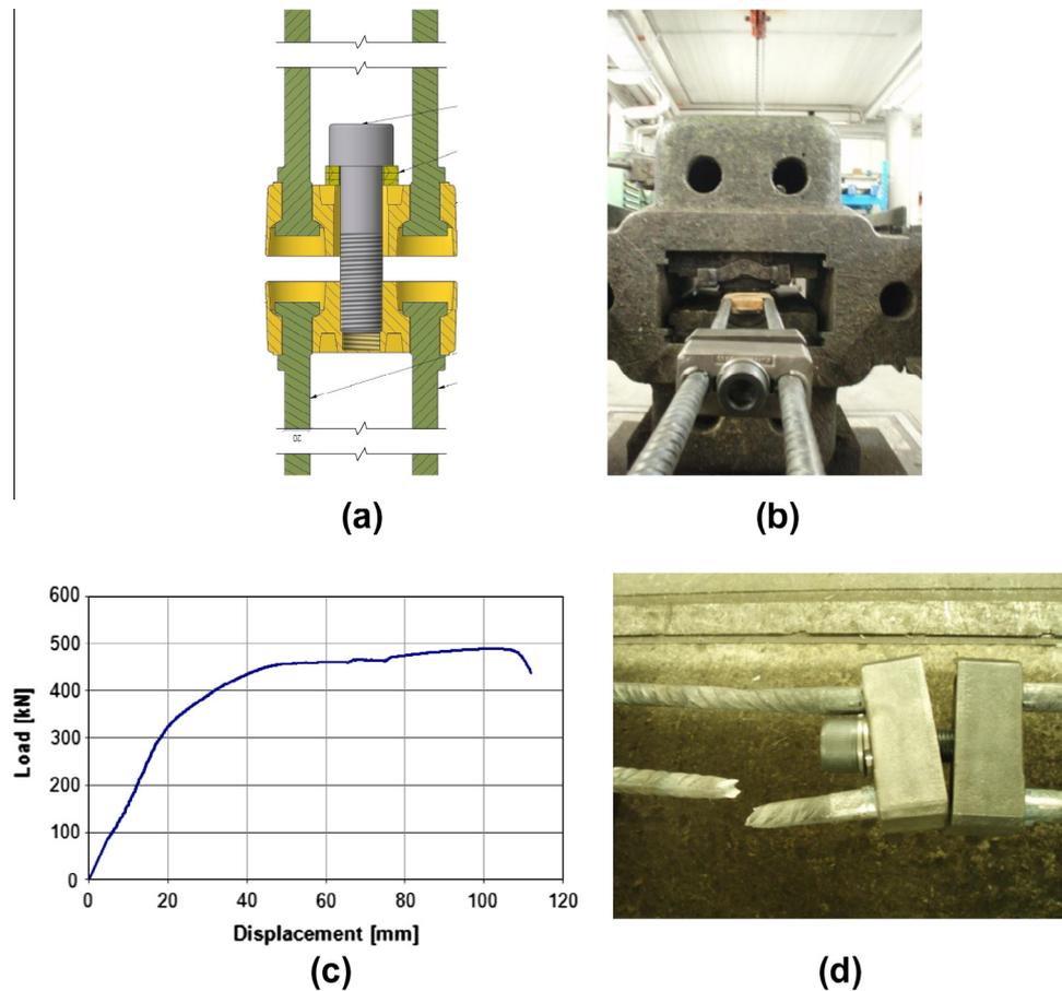
**Fig. 7.** (a) Connector used to realize dry emulative beam–column joints. (b) Test set-up adopted to assess the tensile capacity of the connection system. (c) Typical load versus displacement curve of the bare connection system. (d) Ductile rupture of the longitudinal rebars. Source: [12].
