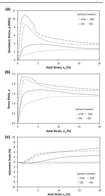
Fig. 2 Experimental triaxial results for sand at 1 MPa confining pressure with a range of Portland cement contents: deviatoric stress (a), stress ratio (b) and volumetric response (c), versus stain [6]
