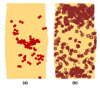
**Fig. 8** Images of the heavily cemented, crushable sample after 4% axial strain. Inner view with all broken fragments highlighted (a), and view of the remaining intact parallel bonds on a vertical cutting plane (b)
