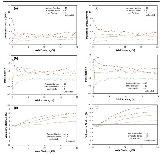
**Fig. 3** Triaxial results for simulations of crushable sand with an increasing degree of cementation: deviatoric stress (a), stress ratio (b) and volumetric response (c) versus strain
